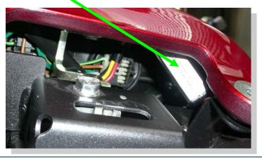
Per the owner's manual, remove the seat and rear compartment to exposes the wire harness.
